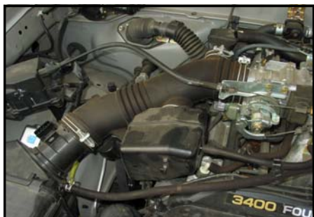
3. At the throttle body, loosen the hose clamps, and disconnect the breather hose on the OEM intake tube.
