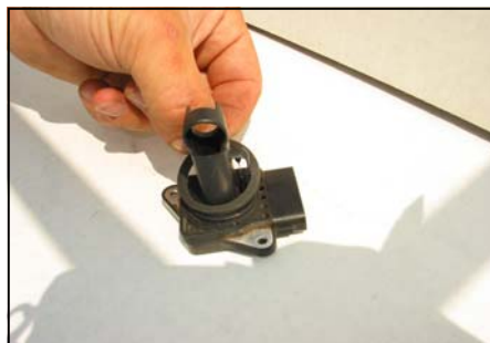
8. Install the mass air sensor to the S&B tube with the original screws
