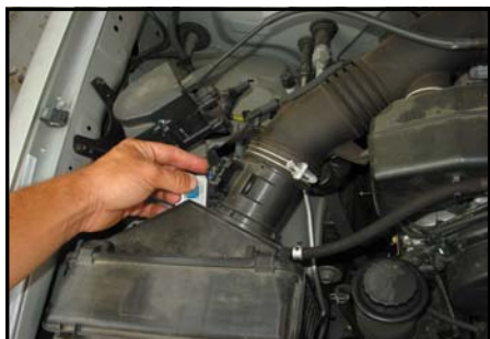
2. Disconnect the hoses attached to OEM air box
