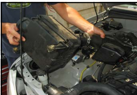
6. Remove the mass air sensor from the OEM assembly
