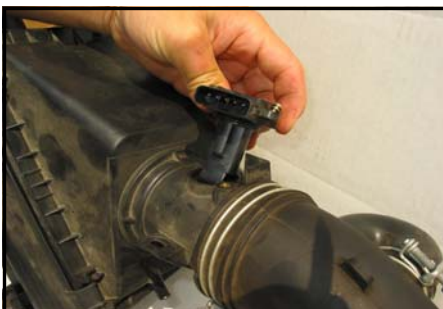
6. Remove the mass air sensor from the OEM assembly
