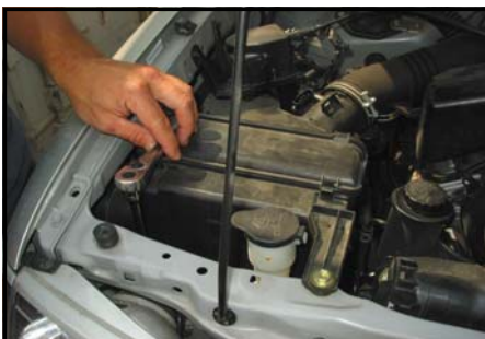
5. Lift and remove the OEM air box and tube from the vehicle
