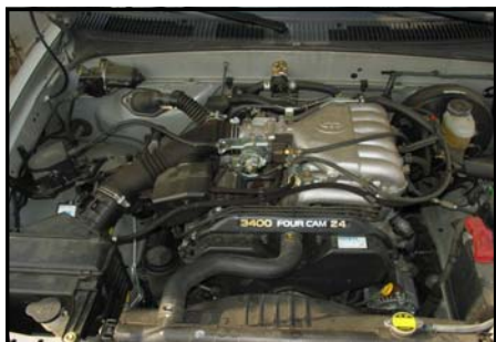
3. At the throttle body, loosen the hose clamps, and disconnect the breather hose on the OEM intake tube.
