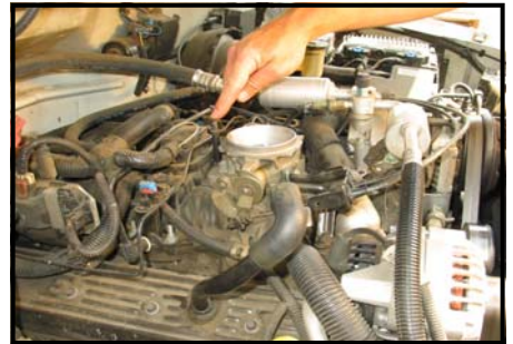
10. Remove the bolt from the stand off using a 7/32" wrench. Take lower portion of the bolt and reinstall in throttle body. Thus, you have just lowered the position of the bolt.
