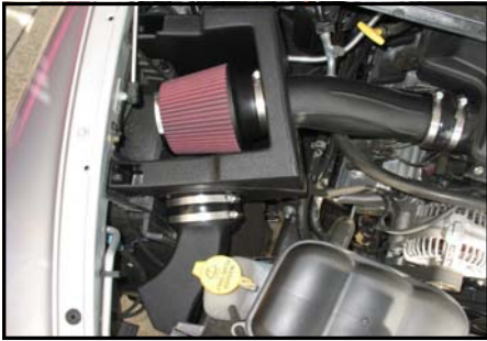
11. Completed Cold Air Intake Kit Installation Picture.
