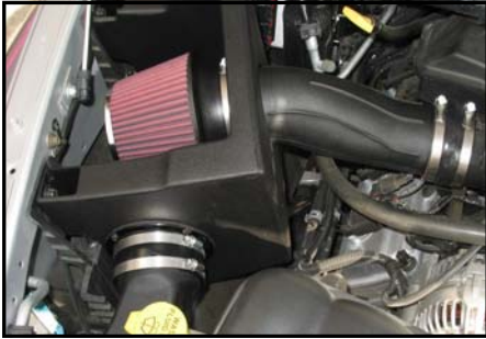
11. Completed Cold Air Intake Kit Installation Picture.
